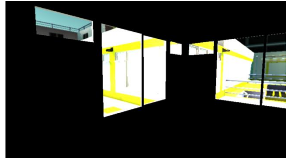
Fig. 15: Contents of the ray traced effect buffer used for reflections
